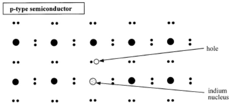
An electron from the next atom can move into the hole created as described previously. Conduction can thus take place by the movement of positive holes. This is called a **p-type semiconductor**, as most conduction takes place by the movement of **positively charged** 'holes'.
