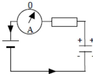
As the capacitor charges a p.d. develops across the plates which opposes the p.d. of the cell as a result the supply current decreases.
