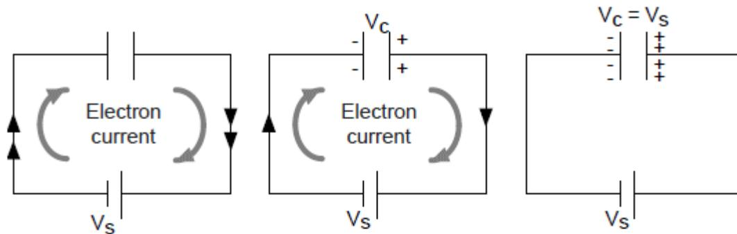
There is an initial surge of electrons from the negative terminal of the cell onto one of the plates (and electrons out of the other plate towards the +ve terminal of the cell).
