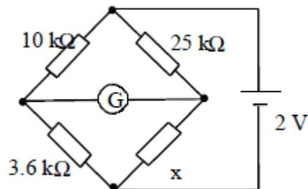
This Assuming the galvanometer (a sensitive meter) has a zero reading we can apply the above equation.
