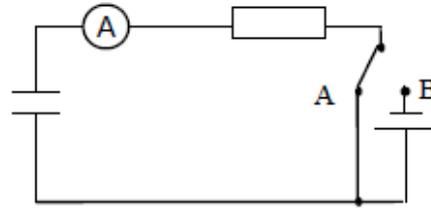
While the capacitor is **discharging** the current flowing in the circuit and the voltage across the capacitor behaves as shown in the graphs below.
