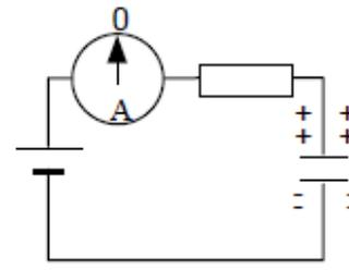
The capacitor becomes fully charged and the p.d. across the plates is equal and opposite to that across the cell and the charging current becomes zero.
