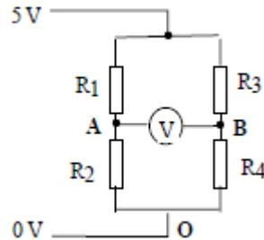
The voltmeter measures the potential difference between the two midpoints of the parallel branches. If the voltmeter reads 0V the bridge circuit is said to be balanced. This will happen when the ratios of the resistors in the circuit are equal.
