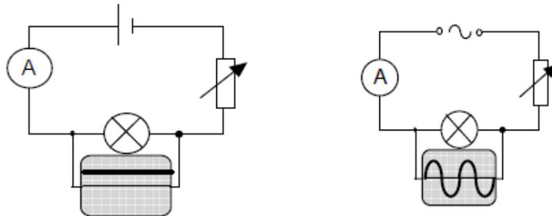
The variable resistors are altered until the lamps are of equal brightness. As a result the direct current has the same value as the effective alternating current (i.e. the lamps have the same power output). Both voltages are measured using an oscilloscope giving the voltage equation below. Also, since  $V=IR$  applies to the r.m.s. values and to the peak values a similar equation for currents can be deduced.
