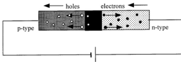
In the reverse biased diode the applied potential difference increases the depletion layer. The diode will become even less likely to conduct.
