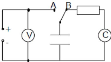
The capacitor is charged to a chosen voltage by setting the switch to A. The charge stored can be measured directly by discharging through the coulomb meter with the switch set to B. In this way pairs of readings of voltage and charge are obtained.
