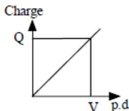
The energy stored in the capacitor is given by the area under graph
