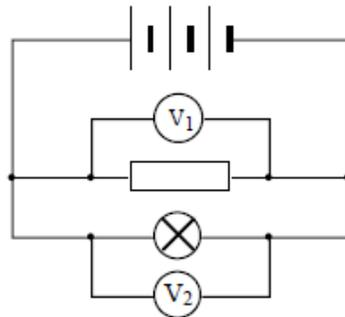
$$V_1 = V_2$$
