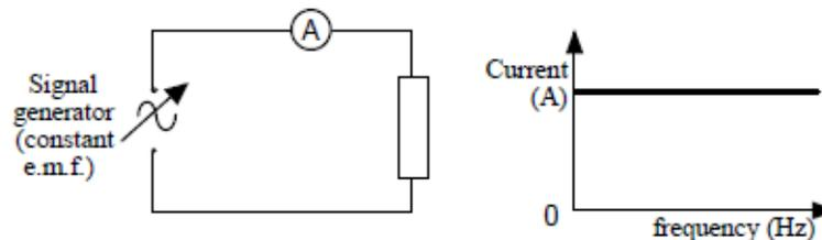
The results show that the current flowing through a resistor is independent of the frequency of the supply.
