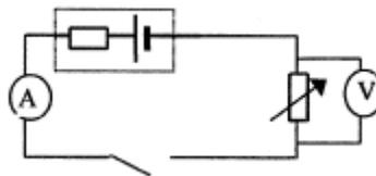
The experimental results show that the maximum power transfer takes place when the resistance already present in the circuit is equal to the load resistance. In the above circuit this happens when  $r = R$ .
