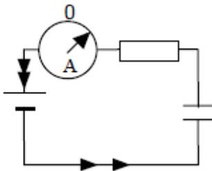
As soon as the switch is closed there is no charge on the capacitor the current is limited only by the resistance in the circuit and can be found using Ohm's law.
