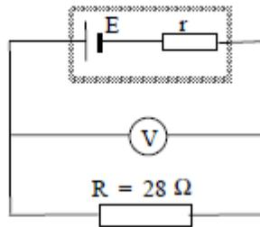
*A cell of e.m.f. 1.5 V is connected in series with a  $28\Omega$  resistor.*
