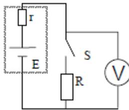
By applying the principle of conservation of energy, the electrical potential energy available from the supply must be equal the energy “wasted” by the internal resistor added to the energy used by the load (external) resistor,  $R$ .
