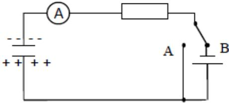
If the cell is taken out of the circuit and the switch is set to A, the capacitor will discharge
