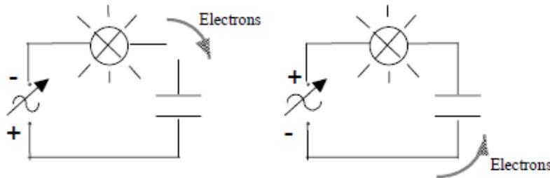
The electrons move back and forth around the circuit passing through the lamp and charging the capacitor one way and then the other (the electrons do not pass through the capacitor). The higher the frequency the less time there is for charge to build up on the plates of the capacitor and oppose further charges from flowing in the circuit. More charge is transferred in one second so the current is larger.
