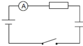
When the switch is closed the current flowing in the circuit and the voltage across the capacitor behave as shown in the graphs below.
