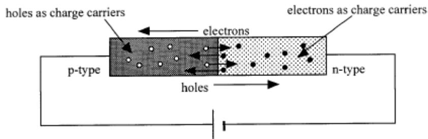
Electrons from the n-type material will be given enough energy from the battery to flow across the junction and round the above circuit in an anti-clockwise direction. This movement will result in a similar movement of holes in the clockwise direction. The diode conducts because the depletion layer has been removed.
