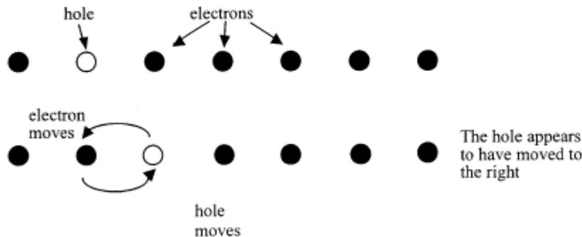
In an undoped semiconductor, the number of holes is equal to the number of electrons. Current consists of drifting electrons in one direction and drifting holes in the other.
