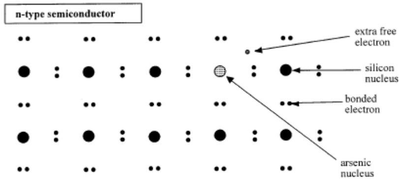
This type of semiconductor is called **n-type**, since most conduction is by the movement of free electrons, which are, of course, **negatively charged**.
