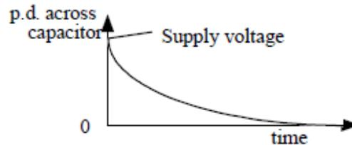
Although the current/time graph has the same shape as that during charging the currents in each case are flowing in opposite directions. The discharging current decreases because the p.d. across the plates decreases as charge leaves them.
