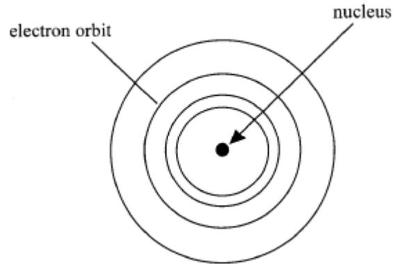
In insulators the outermost level has no electrons that are free to move. In conductors the outermost level does have electrons that are free to move which allows electrical conduction to take place.
