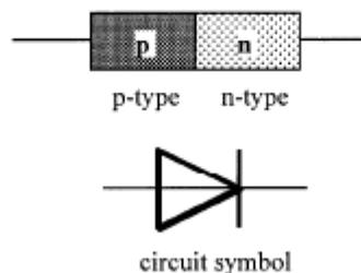
Some of the free electrons from the n-type material diffuse across the junction and fill some of the holes in the p-type material. This can also be thought of as holes moving in the opposite direction to be filled by electrons. This movement means the area around the junction loses virtually all of its free charge carriers. This area is therefore known as the depletion layer.
